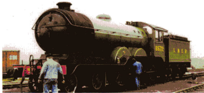
The M&GN Joint Railway Society's Class B12 no. 8572 was built in 1928 for LNER express services to East Anglia. The only working inside-cylinder 4-6-0 loco in Europe returns to the Poppy Line in 2010 after a major overhaul.
